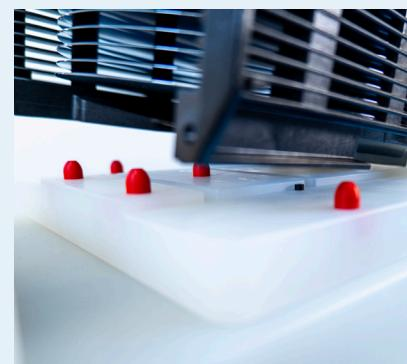
exchange when integrated SEND and RECEIVE stage cassette-in-place sensors are activated. An adjustable transfer arm resistance sensor to detect excessive forces during motion—safeguarding wafer integrity.
